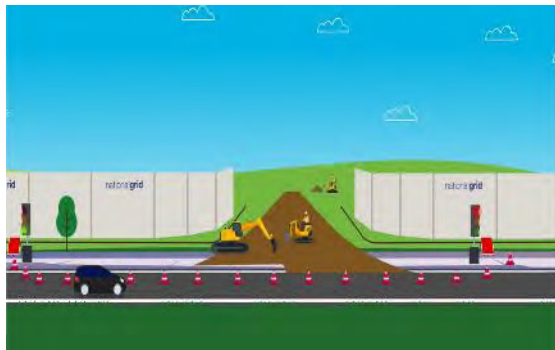
Step 2 The soil is stripped to a depth of at least 1 metre. Any services in the verge would either be diverted or worked around
