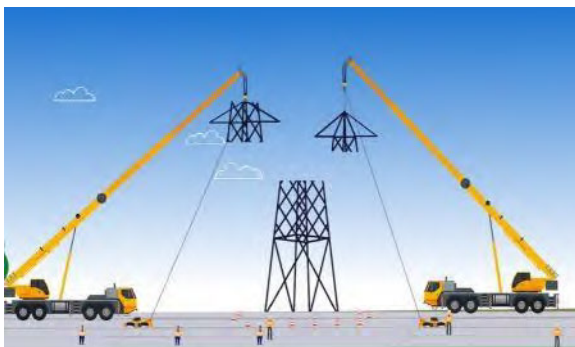
Step 3 Pylon sections are removed using cranes (felling) and the steel is taken off site to be recycled
