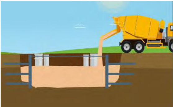
Step 3 The pile foundations are built and kept in place with pile caps which the legs of the pylon sit on top of
