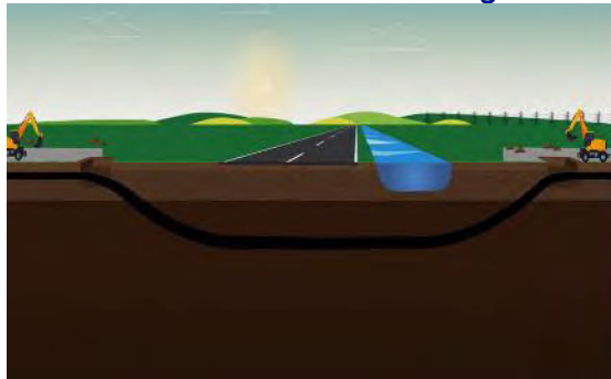
Step 5 Once complete the above ground sites are reinstated and the site access removed
