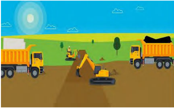
Step 1 The topsoil is stripped from the land where the road would be built
