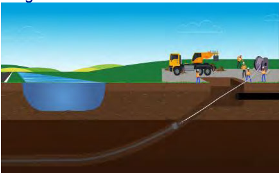
Step 3 A wire called a bond is attached to the drill and is pulled back to the other side of the works
