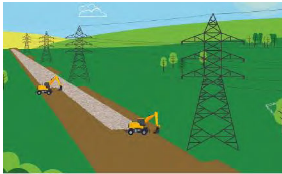
Step 6 Once everything has been checked, the site access is removed and land reinstated as per agreement with the landowner
