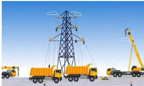
Step 2 The wires and insulators are removed by winching the equipment to the ground
