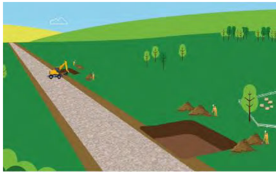
Step 2 The area is cleared at each pylon site to create a working area
