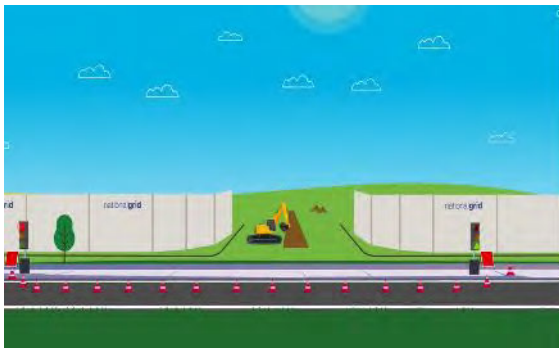
Step 1 Safety measures including hoarding where needed and traffic management are installed prior to works beginning
