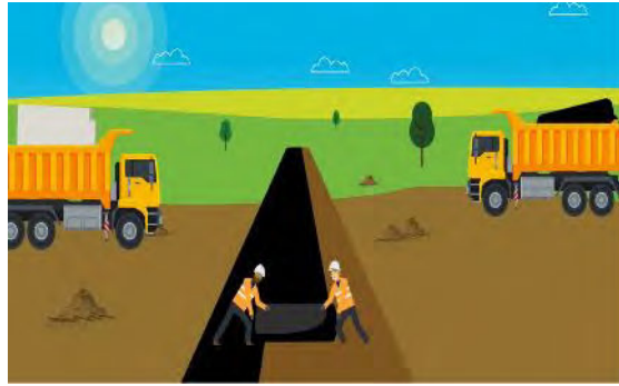
Step 2 A layer of synthetic material is installed to allow water to filter through the service, and protect the subsoil from the stone laid for the road surface
