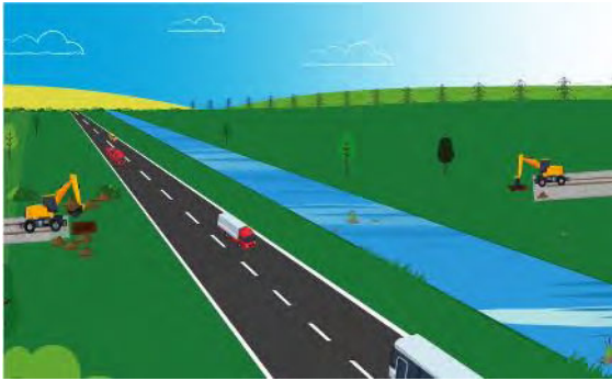
Step 1 The topsoil is removed for the temporary site access and two pits are dug either side of the section of cable
