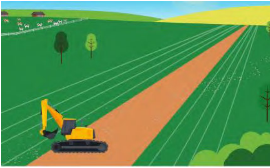
Step 1 Cables are installed in six trenches, adjacent to the temporary site access
