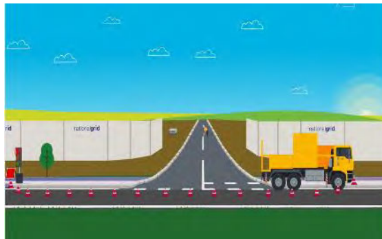
Step 6 Road markings (for permanent bellmouths) are painted and traffic signs installed as per agreement with the local highways authority
