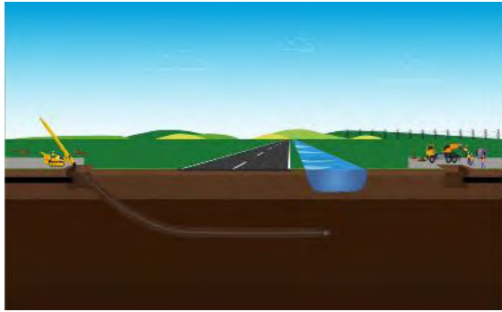
Step 2 From one pit a drilling machine that drills beneath the obstacle to the other side is launched
