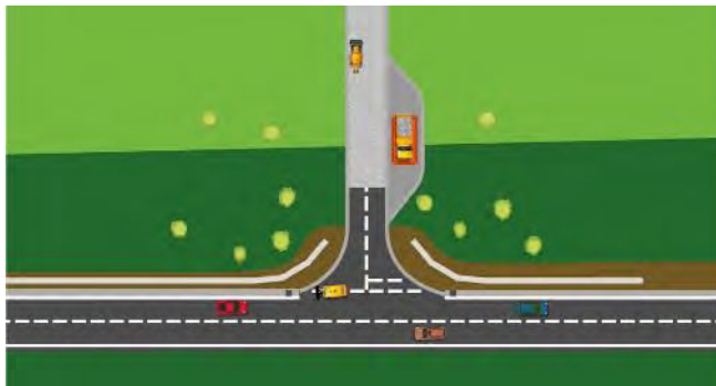
Step 5 Wheel washes are installed to ensure dust and soil from site does not leave
