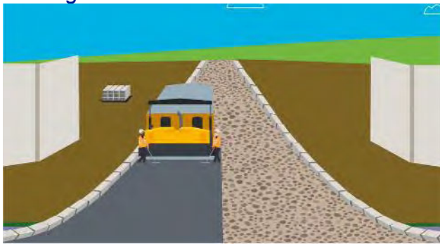
Step 5 A suitable, durable layer of material is laid as the final road surface
