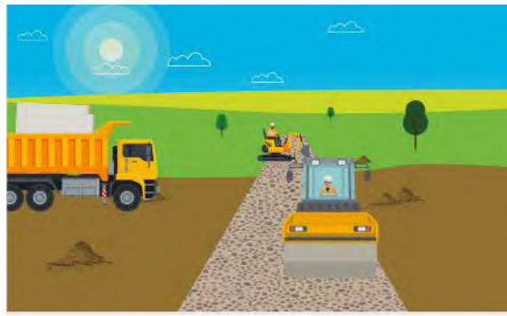
Step 4 The road is then rolled and topped with a layer of smaller stones which vehicles can drive over
