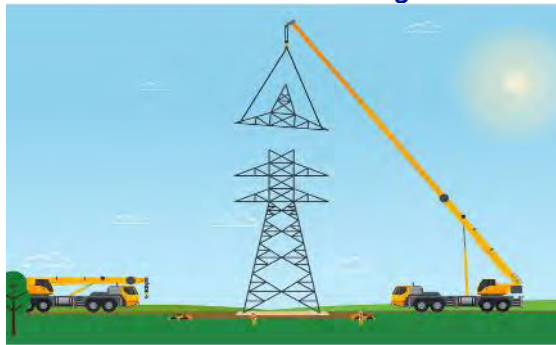
Step 4 The pylon is lifted into place in four parts
