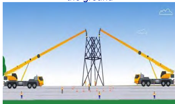
Step 4 The remaining structure is secured in place whilst the legs are cut and the pylon is lowered safely to the ground and dismantled
