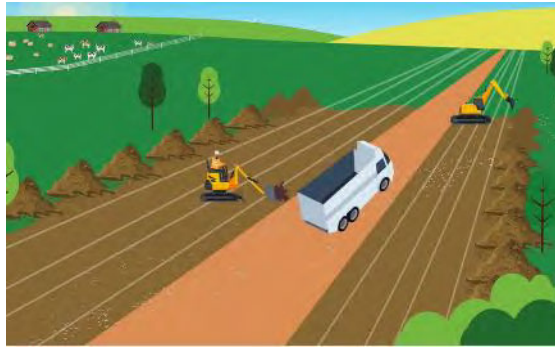
Step 2 The topsoil is removed and stored alongside the trenches so it can be put back after the work is complete
